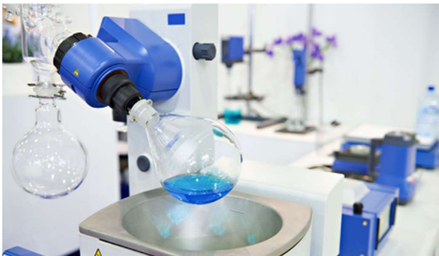
Reagent concentration by evaporator
