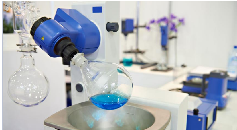
Reagent concentration by evaporator
