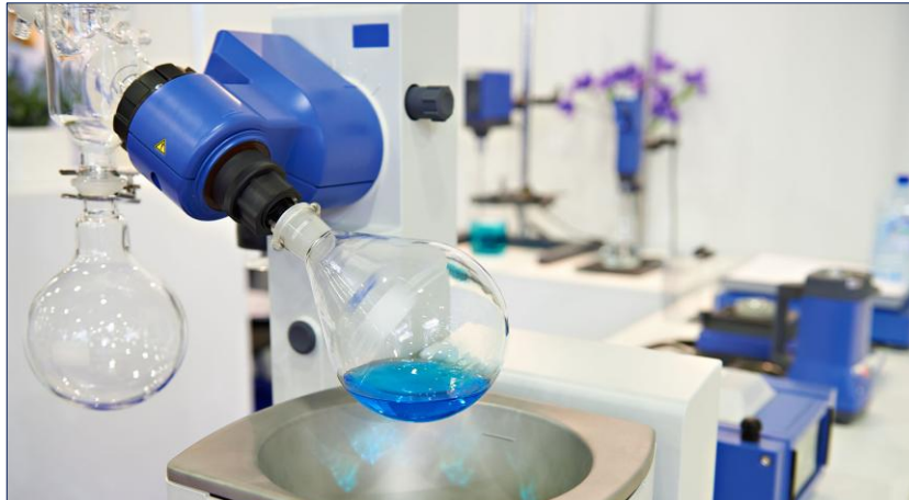
Reagent concentration by evaporator
